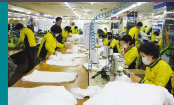
3단계 : 봉제(본봉미싱 작업순서:밑단-라벨부착) Sewing (sewing machine sequence : tail edge - label attached)
